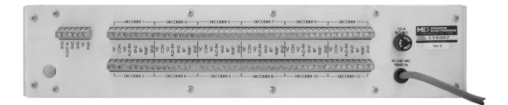
The terminal blocks are in groups of 8 inputs, with each group associated with one of the 3185E cards installed. NC is the normally closed contact on the 3185E board, NO the normally open contact, and the COM terminal s the common of the relay contacts. SET, when momentarily pulled to GND, turns ON the 3185E card, closing the relay.
